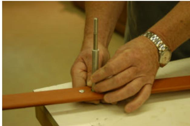
Next, insert the bolt up through the long arm bearing.
