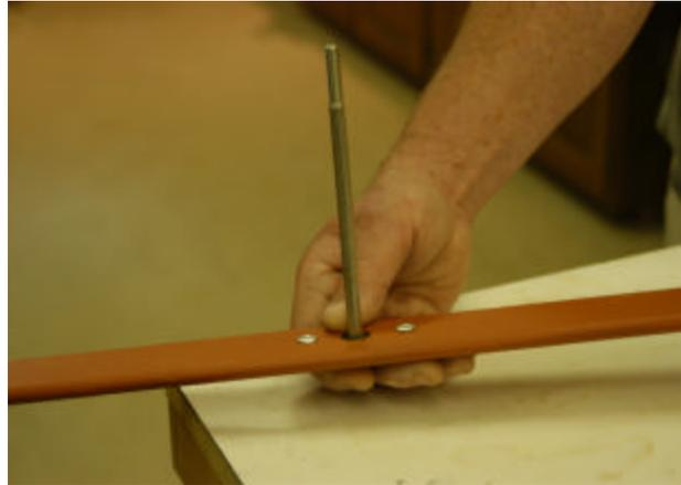
Slide the long 3 1/4" aluminum sleeve onto the bolt.
